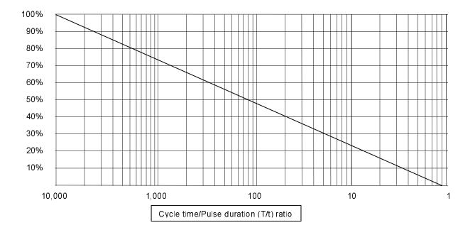
For improved performance and reliability, a 30% pulse derating factor is recommended (50% if parts are subjected to multiple pulses)... Always verify selection by evaluating prototypes under worst-case conditions.
