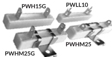
Designed for general purpose and semi-precision power applications, the ceramic construction is fireproof and resistant to moisture & solvents. The internal element is wirewound on lower values, power film on higher values, depending on size and options (**Opt. P** parts are always Wirewound). If a specific construction is preferred specify **Opt. WW** for Wirewound, **Opt. M** for Power Film (not available in all values).
